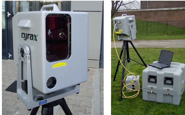
Figure 1.4. Leica HDS 2500 time-of-flight laser range scanner. Maximum image dimensions: 1000 \times 1000 . Maximum range: 100m. Maximum field of view: 40^\circ . Positional accuracy: \pm 6\text{mm} (1.5 to 50m). Distance accuracy: \pm 4\text{mm} . Angular accuracy: \pm 12'' . Beam spot size: 6mm (0 to 50m).
