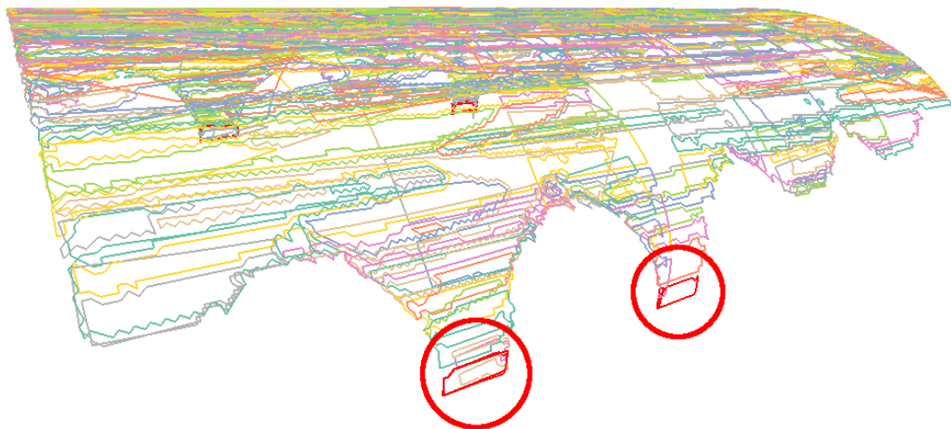
Figure 5.4. Merging with invalid boundaries flagged. The shape of a component sometimes precludes projection to a flat parameter space without spoiling the topology by folding over. We detect surface self-intersection by testing boundary for curve self-intersection.
