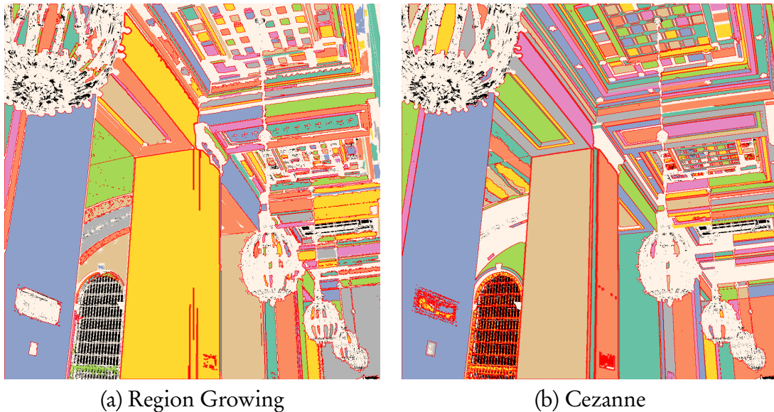
Figure 4.19. Segmentation results: Region Growing vs. Cezanne. Black denotes holes where the scanner failed to register. Nonplanar areas are colored white. Eight other colors are assigned randomly to differentiate the planar regions, and each region is outlined in red. (a) Region growing produces components that are not necessarily planar, such as the large yellow column in the foreground. (b) Cezanne is less likely to be confused by local aberrations.
