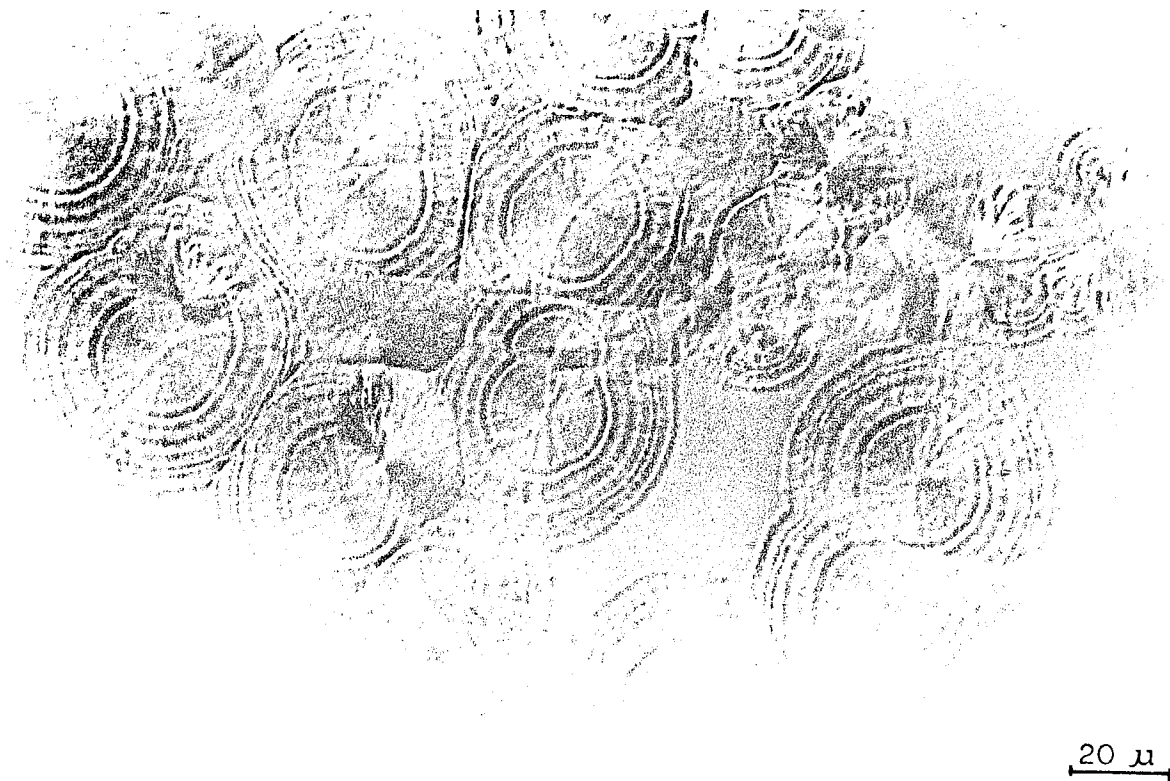
Fig. 31. Optical Micrographs of Thin Films Made by the Evaporation of 1% (w/v) TPI Amyl Acetate Solution
