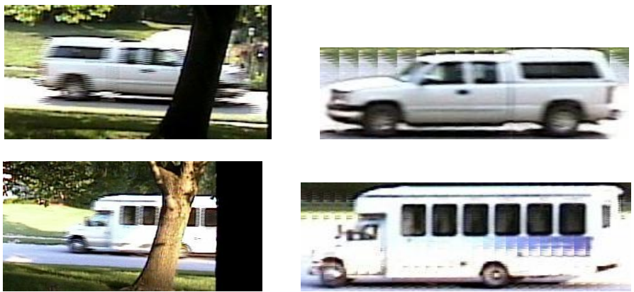
Figure C.4. Examples of a pickup and a transportation bus. Original image shots on left, reconstruction results on right
