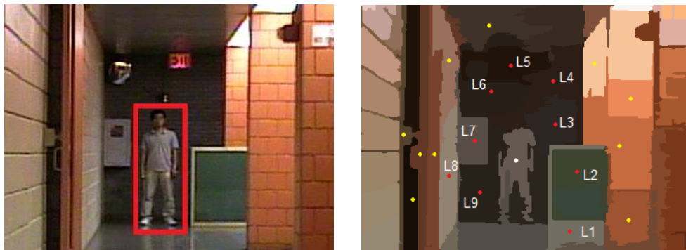
Figure 3.11 Surface selection in a segmented image of a 31 meters corridor.
