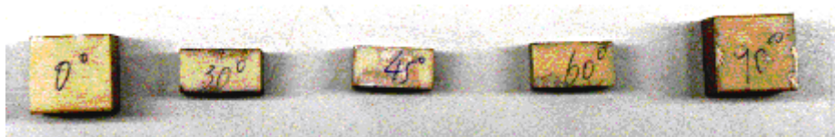
Fig 4.3 Five small samples with different angles to the poling direction
