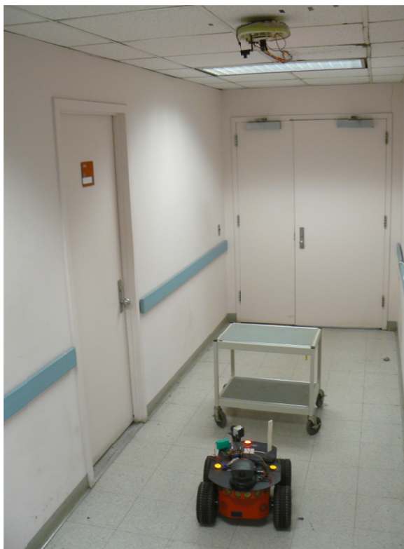
Fig. 3.4 shows an experimental setup of the dual-robot system consisting of a ground robot and a wall-climbing robot operating on the ceiling to map the indoor environment.
