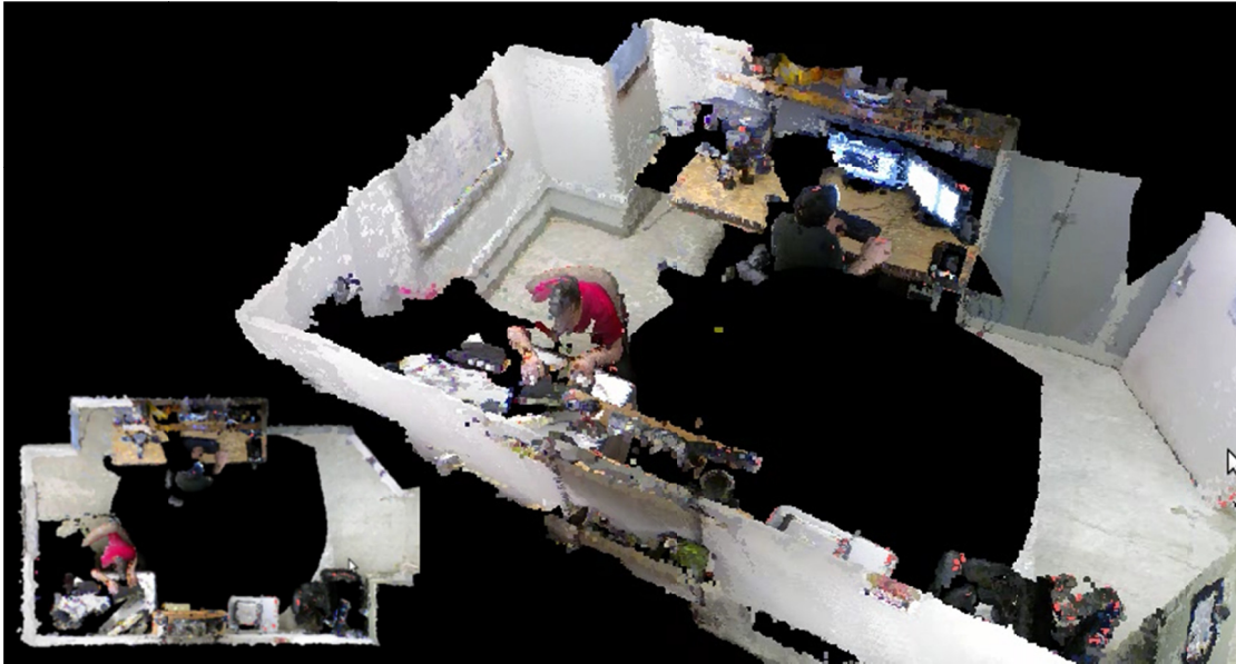
Fig. 7.6 3D map of an office built by rotating the RGB-D camera - side view and orthogonal top view.
