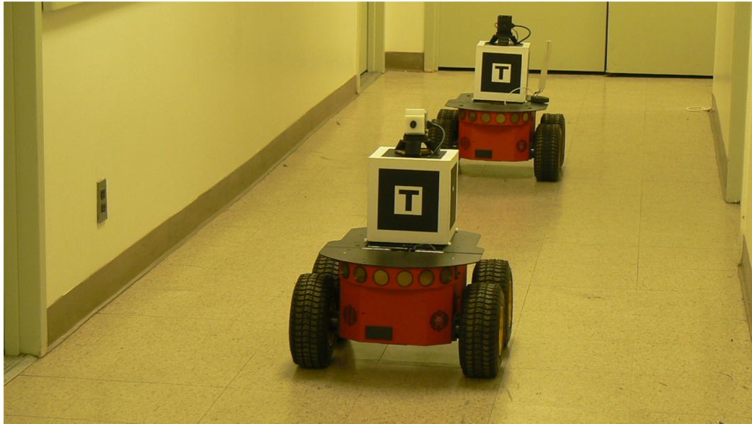
Fig. 4.1 Two Pioneer® ground robots mapping the indoor environment using the vision-aided laser mapping algorithm.
