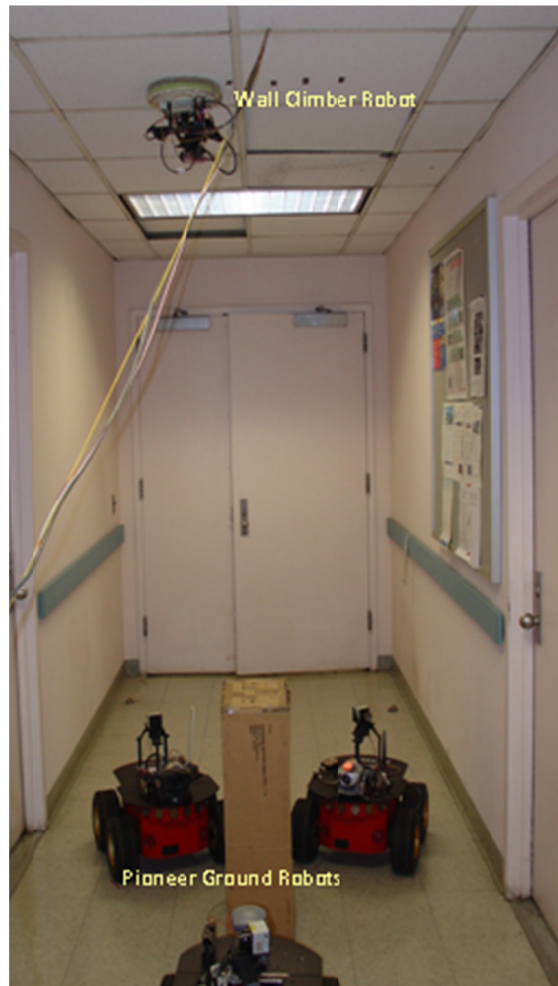
Fig. 3.1 shows experimental setup that includes three ground robots and a wall-climbing robot on the ceiling.
