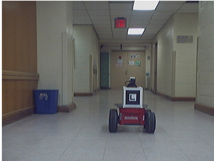
Fig. 5.11 Setup shows a ground robot acquiring a 3D range image in an office corridor.
