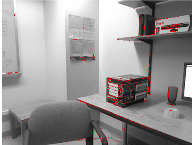
Fig. 7.2 Outcome of brightness edge feature extraction algorithm on a single RGB-D frame acquired by the Kinect® sensor in an indoor environment.
