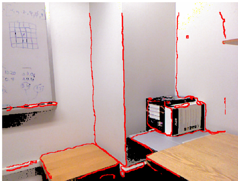
Fig. 7.5 Edge features extracted using mode-histogram morphology on local normal vectors computed from a RGB-D frame. The red markings are overlaid on RGB frame acquired by the RGB-D Kinect® sensor.
