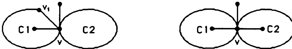
(a) Contract the edge between v and v_1 and add a pendant edge at v .
