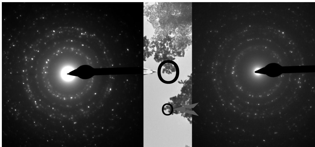
Figure 2.4. \mu D pattern images displayed on a monitor corresponding to unknown NP aggregates that were identified as ZnO by Method 2 (overhead transparency method).
