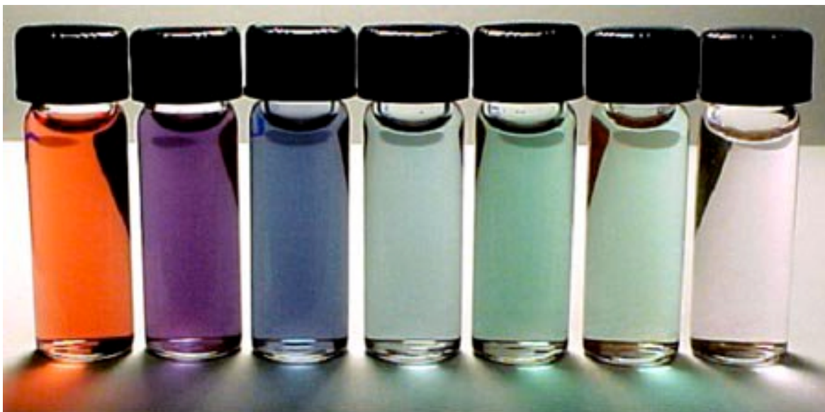
Figure 1.2. Gold colloids exhibit different colors in relation to different particle sizes. The larger the NP size, the more red-shifted wavelength it absorbs, and the more blue it appears. (Picture taken from http:// beforeitsnews.com/story /104/900/NanoGold_ Revolution:_Alchemy _of_ the_21st_ Century.html )
