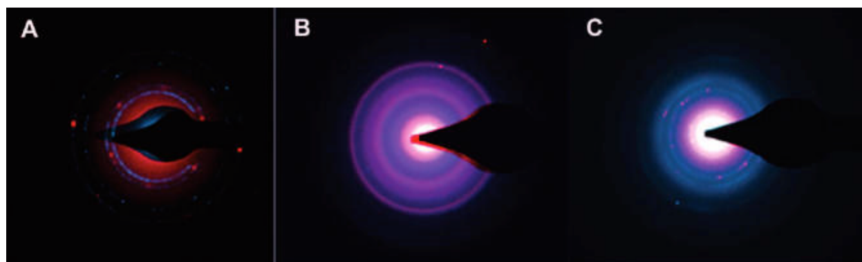
Figure 3.5. ED patterns in red of the prepared nanodiscs of (A) gold, (B) nickel, and (C) cobalt. The corresponding standards are superimposed and are in blue.
