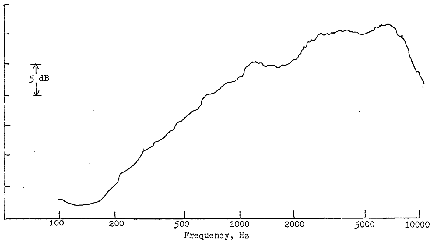
Fig. 11. Real time spectrum analysis: frequency response of +6 dB/octave. White noise was passed through channels 1 and 2 combined. Channel 1 was set to a bandwidth of 125 Hz to 1000 Hz, and channel 2 was set to a bandwidth of 1000 Hz to 6000 Hz. Compression ratio was 1:1.
