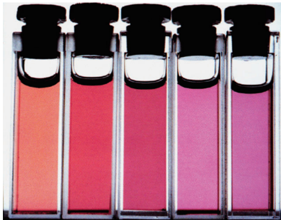
Figure 1.9 Change in color of gold nanoparticles where refractive index of dielectric surrounding is changed from lower to higher index (Left to right). [17]
