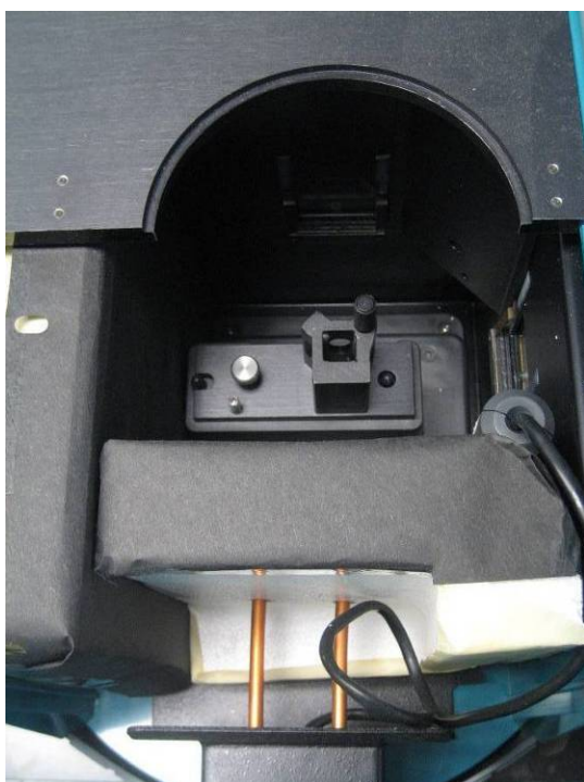
Figure 22. Modified interior for LT Fluorescence (Shown with cuvette holder, Dewar housing not pictured).
