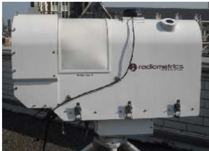
Figure 5.2: Microwave Radiometer, Model: MP-3000A.
