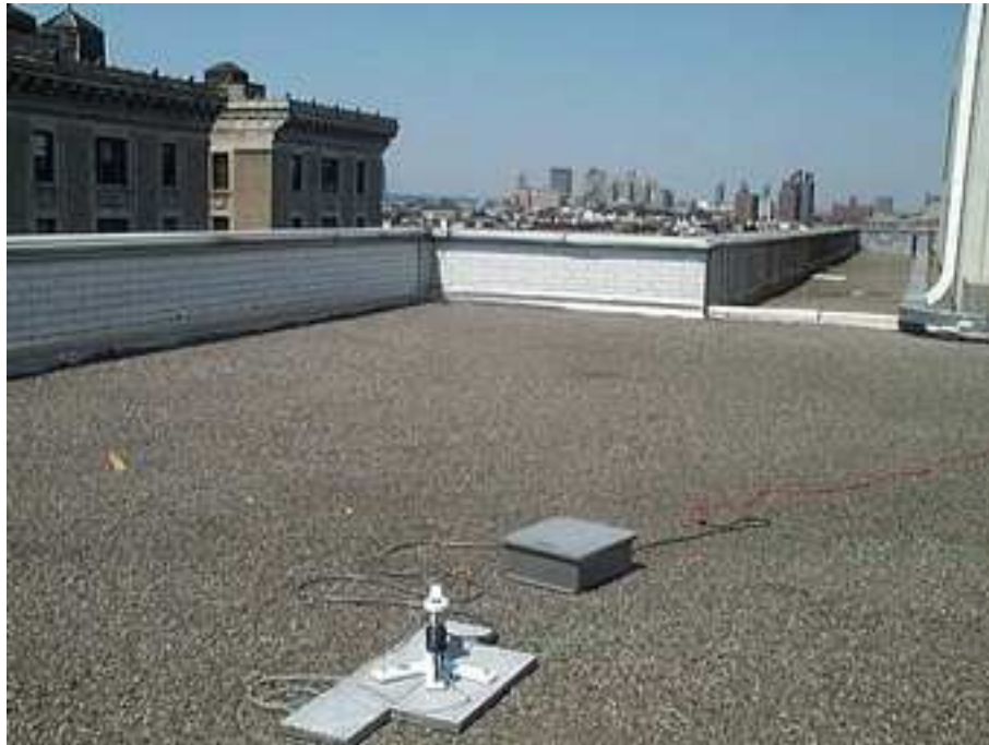
Figure 3.3: The CIMEL sun photometer mounted at City College of New York (CCNY in AERONET).
