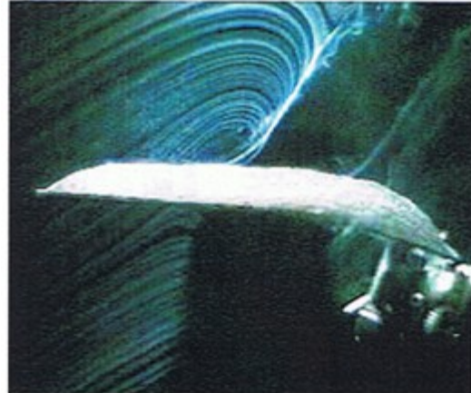
Fig. 3.8 Unsteady leading edge vortex as seen from behind and below a MAV wing [47]
