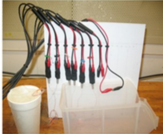
Fig. 5.23 Calibration of thermocouples with ice water
