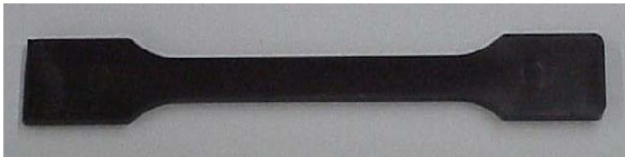
Figure 5.2: The tensile test dog bone specimen
