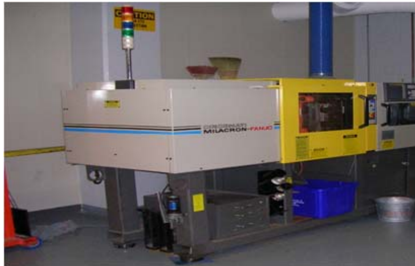
Figure 3.1: Robo 55R-22 reciprocating screw injection molding machine
