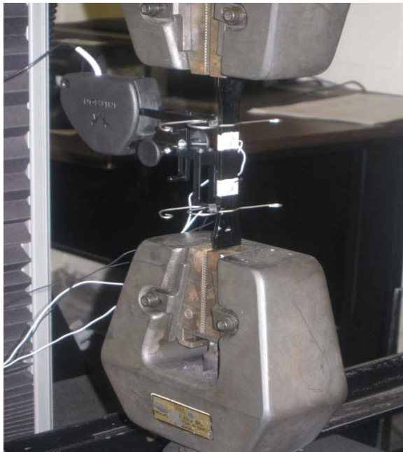
Figure 6. 1: Specimen in the INSTRON machine with the extensometer and the electrical probes.
