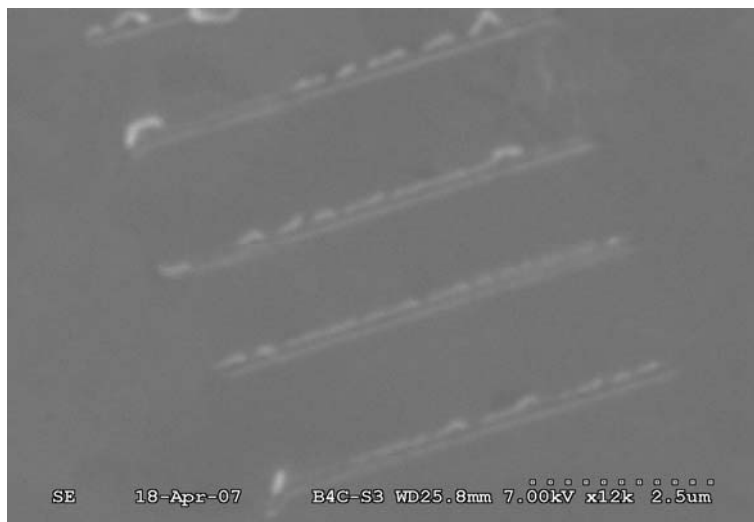
Figure 9.7 Gold array formation on the patterned area after the gold solution was reduced by sodium borohydrate ( Nurxat, Linglu, & Kai)
