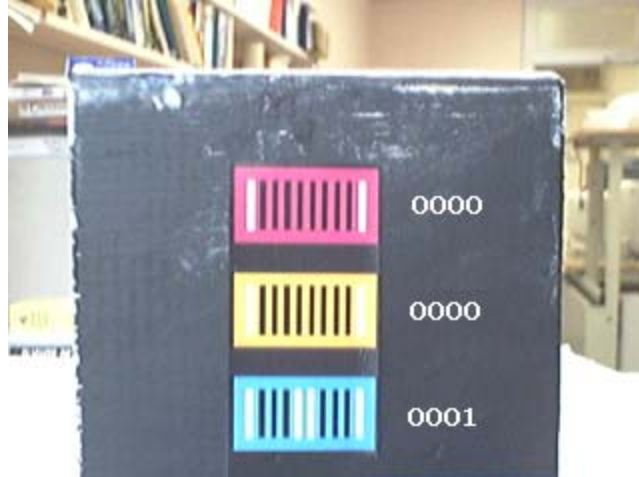
Figure 4.6: Each barcode color represents a specific attribute. The number encoded by the barcode represents the value of that attribute for this object.
