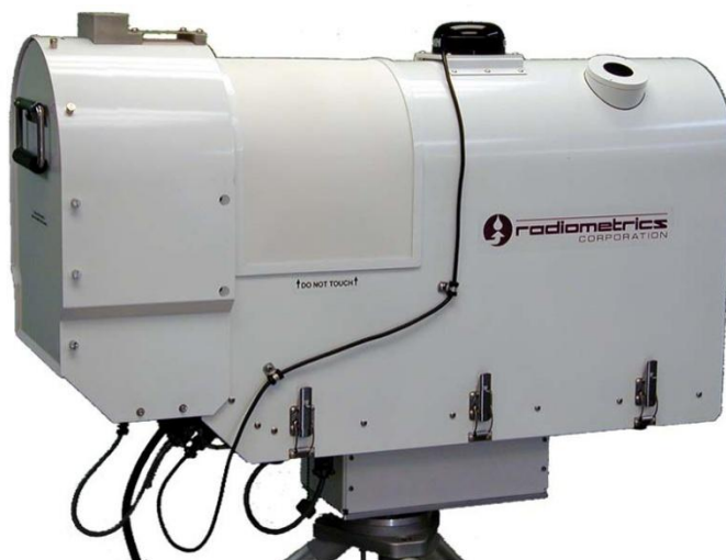
Figure 2.10: MP-3000A Hyper-Spectral Temperature, Humidity and Liquid Water Profiler.
