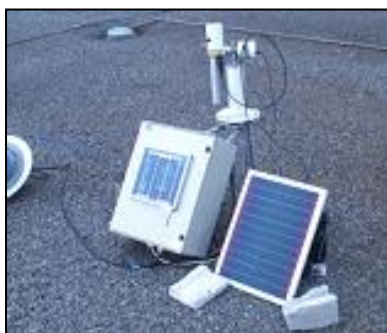
Figure 2.9: Sunphotometer (CIMEL Electronique 318A spectral radiometer) located at CCNY
