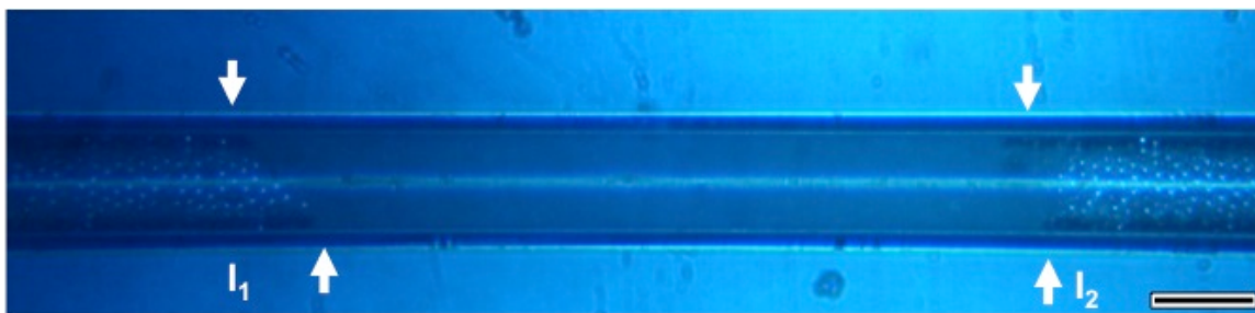
Figure 3.3 Optical microscope image of 50 mm PMMA capillary filled from left to right with 10 \mu\text{m} , 2.5 \mu\text{m} and 10 \mu\text{m} showing tilted interface I_1 and less angled interface I_2 . White arrows indicate the interfaces at the upper and lower side of the fiber. Scale bar 50 \mu\text{m} .
