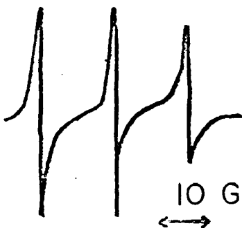
Figure 8. ESR spectrum for spin trapping during polymerization of N-methyl methacrylamide.
