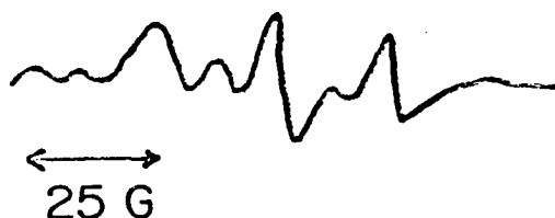
Figure 1. ESR spectrum of irradiated PMMA at 300°K.
