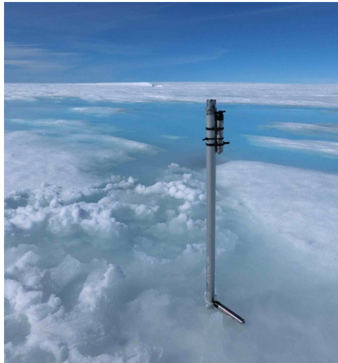
Figure 4-1 Configuration of the top and bottom pressure transducers deployed at lake Ponting on June 13 th , 2011. The aluminum pole was drilled into the ice down to 3m. The difference between the heights of the two sensors is 0.7 m.
