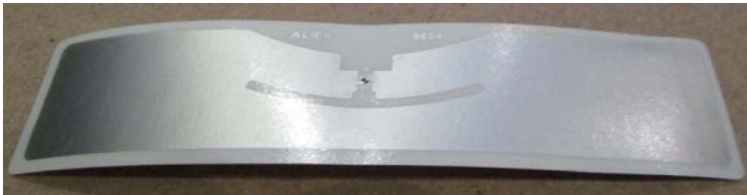
Figure 6.3: Backside of passive Alien type G RFID tag (ALN-9654)
