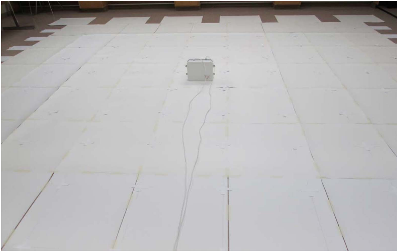
Figure 6.6: Testing region with 144 pairs of RFID tags (half meter apart)
