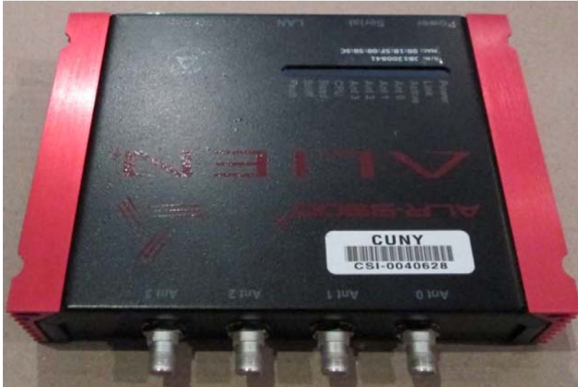
Figure 6.2: RFID reader of Alien Technology (model number is ALR-9900+)
