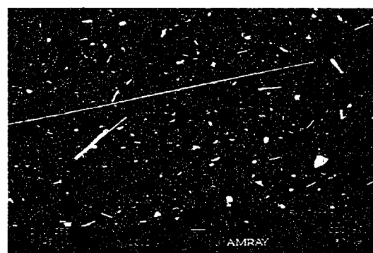
Figure 11. SEM image of MCE filter surface showing particles and filter's texture.
