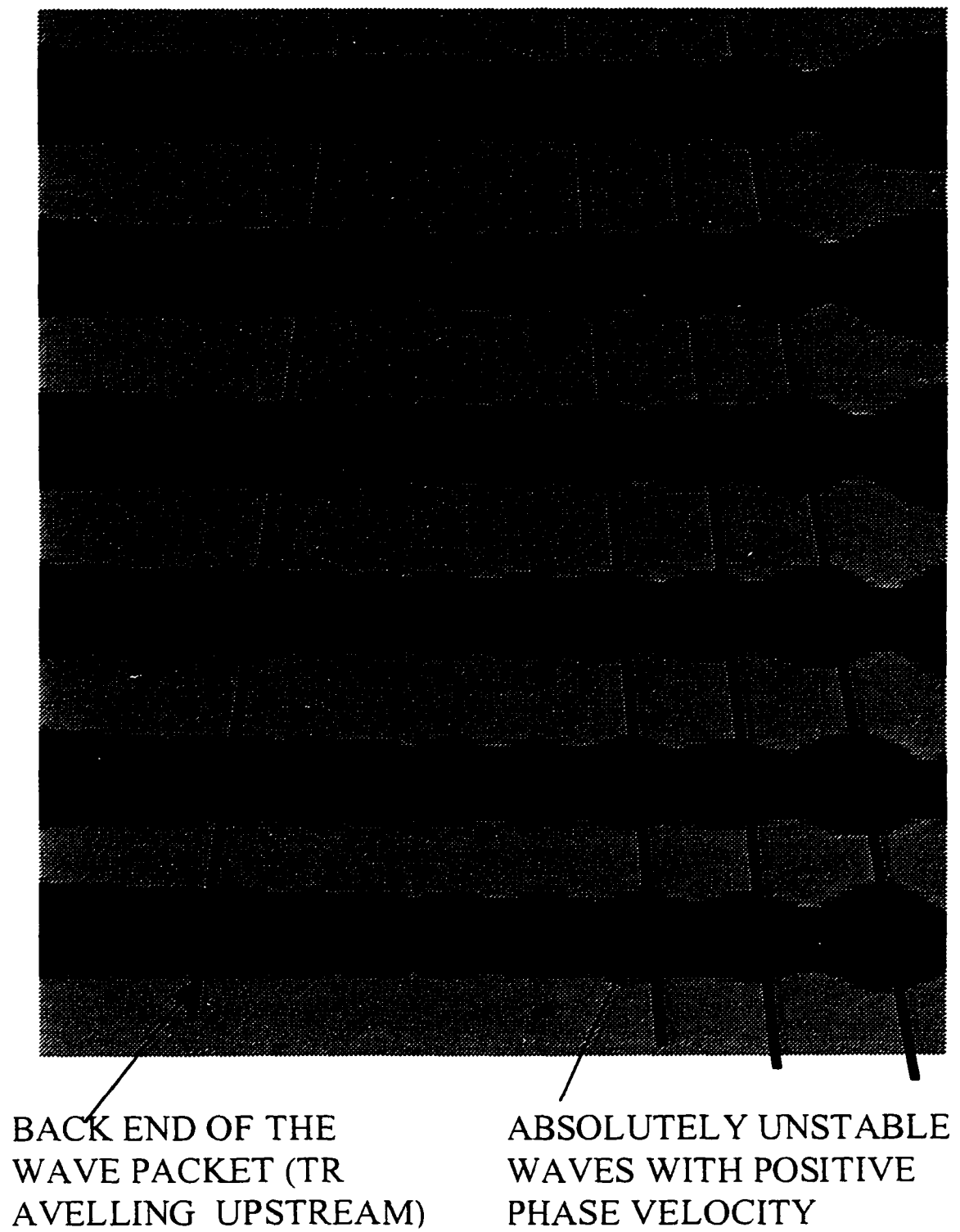
Figure 1. Upstream propagating modes at Weber number below the critical
