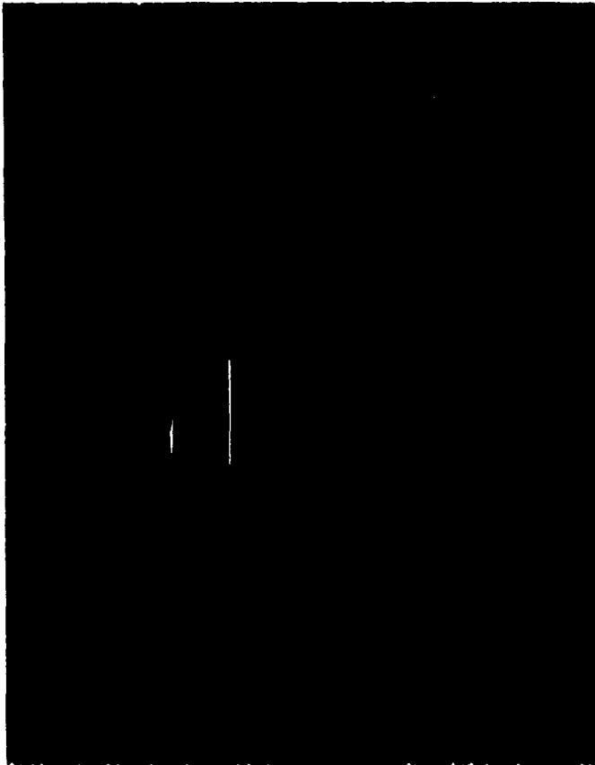
FROM LEFT TO RIGHT: 4500 Å, 4358 Å, 4078 Å, AND 4047 Å FIGURE 3.6:4 SPECTROMETER PHOTOGRAPH OF THE 4500 Å LASER LINE FOR SEQUENTIAL OPERATION
