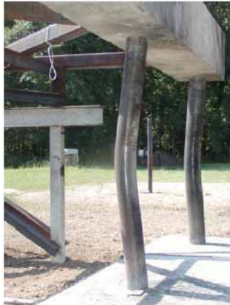
Figure 6.17: Plastic Hinge Formation in a Pier During Blast Test by Bruneau et al. (2006).
