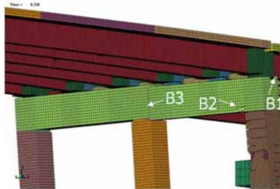
Figure 6.18: Damage Mechanisms for the Failure of the Bent Beam.
