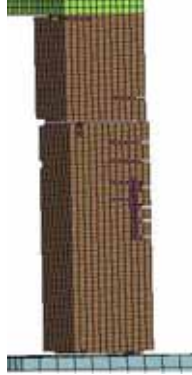
Figure 6.16: Formation of Plastic Hinge in the middle of a Pier.
