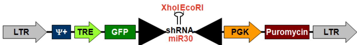
Figure 5: Map of doxycycline-inducible construct for shRNA expression. shRNA oligos for mdm2 , mdmx or p53 were inserted between XhoI and EcoRI restriction sites. GFP expression was used to assess shRNA expression.
