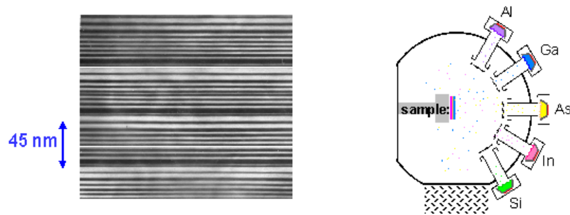
Figure 2.9: Micrograph of a cross section of a QCL with several stages of active and injector layers and MBE process [18]
