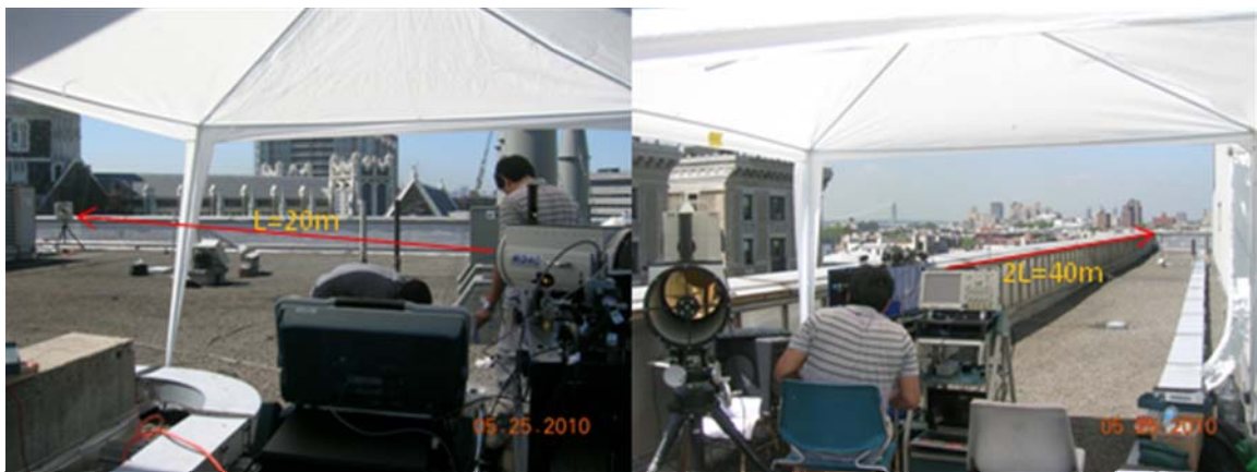
Figure 4.19: Photos of two systems (QCLOPS and OP-FTIR) describing system telescopes and light source/retroreflector positions with optical path-lengths
