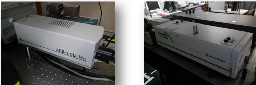
Fig. 3.5 532 nm CW-Nd: vanadate Laser (Millennia Pro, Spectra Physics, left) and Ti:sapphire oscillator system (Tsunami, Spectra Physics, right). The broad band tunable Ti:sapphire oscillator is pumped by the 532 nm CW-Nd: vanadate laser. The system delivers 100 fs, 800 nm laser pulses with a repetition rate 82 MHz.
