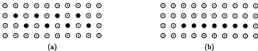
Figure 2.8: Which skeleton is “appropriate” for an n \times 4 object? A point marked \odot is originally a black point but deleted by a thinning algorithm.
