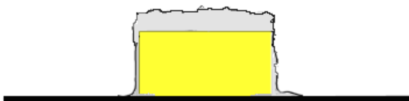
Figure 4.6 Schematic representation of wide gold-insulated nanowire (10-25 μm). Because of the large structure the polymer interlayer is incomplete. However enough polymer intercalates between the gold and the substrate to bind the metal film on the surface. The thickness of the polymer sidewalls are not drawn to scale and are anticipated to be incomplete films.
