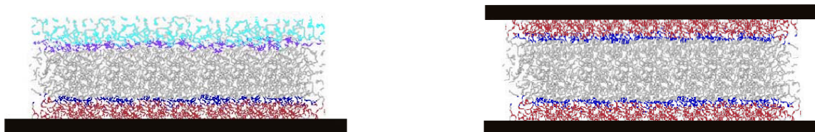
Figure 5.6 Schematic of the three-layer model used to describe the behavior of thin polymer films at interfaces. Left: Substrate supported thin film. Right: Film confined between two substrates. Red: dead layer which has chain mobility strongly influenced by substrate. Gray: bulk-like layer which has the same mobility as that of the bulk samples. Light blue: liquid-like layer, at the polymer-air interface, with higher mobility. Dark blue: interfaces between these layers.
