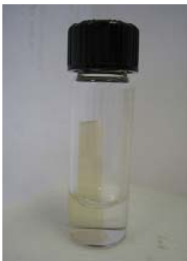
Figure A2.13 4.5 \text{ cm}^2 of mica with a film formed by eight deposition cycles shows no desorption in 1 mL of \text{H}_2\text{O} after 20 days.
