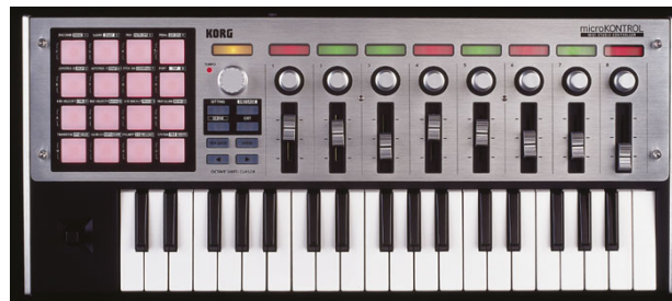
Figure 1.3: Korg MicroKontrol, the type of MIDI keyboard used by Kerpel when writing Charangueando . Note the finger pads used for percussive input, as well as the faders, dials, and buttons that may be assigned to various mixing and recording parameters. This controller is ideal for Kerpel, as it combines recording and performance functionality. (Image courtesy of Korg USA)
