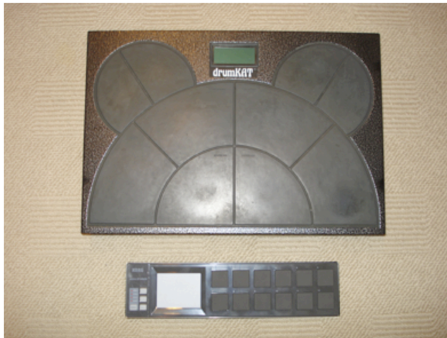
Figure i.13: DrumKAT (top) and NanoPad (bottom) MIDI percussion controllers
