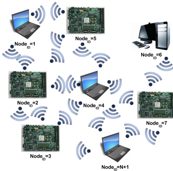
Figure 5.10: Wireless ad hoc network topology in testbed using FPGA devices, laptops, and desktops
