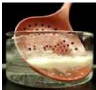
Figure 3.10. Scooping out a thin-layer of diesel gel from the top of water
