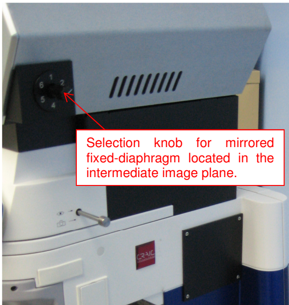
Figure 4.1: Selection knob located on the right side of the CRAIC Technologies Inc., QDI 2010 microspectrophotometer used to position one of six fixed-diaphragm mirrored specimen image mask.
