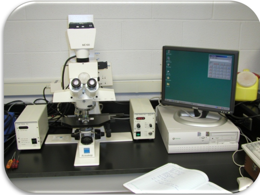
Figure 3.3: Zeiss MPM400-MSP65 Visible Microscope Photometer and Microscope System Processor. This original image was obtained by Dale K. Purcell during performance evaluation on June 19, 2012.
