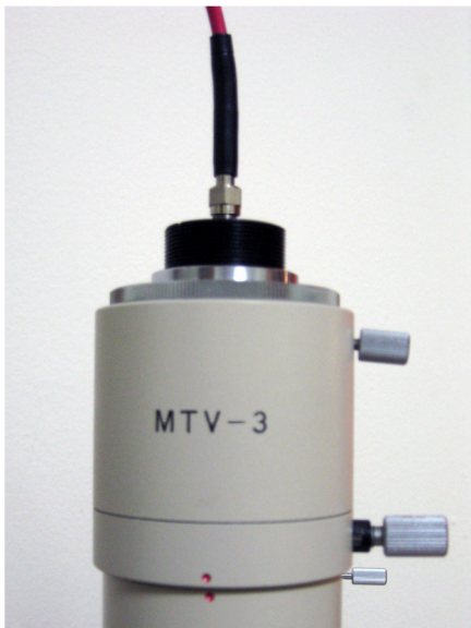
Figure 4.5: Fiber optic SMA connection via an Olympus MTV-3 with a 3.3x NFK photo relay lens connected to an Olympus BH-2 series trinocular head. The SMA adapter is capable of being vertically adjusted inside of the outer black ring order to bring the tip of the fiber optic into sharp focus in the intermediate image plane, which is confocal to the specimen plane.
