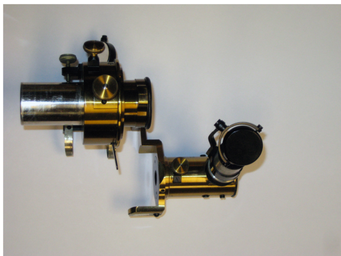
Figure 2.1: Sorby microscope spectrograph. This spectrograph is on display at Microtrace LLC, 790 Fletcher Drive, Suite 106, Elgin, Illinois, 60123.
