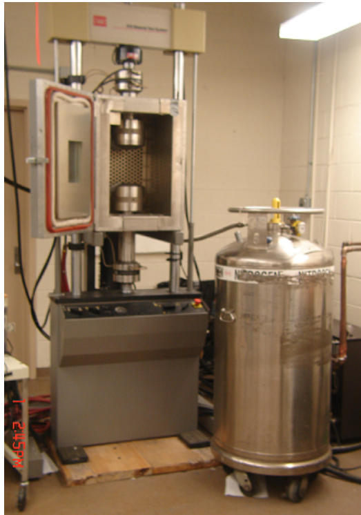
Figure 3.4 MTS machine with environmental chamber and liquid nitrogen tank
