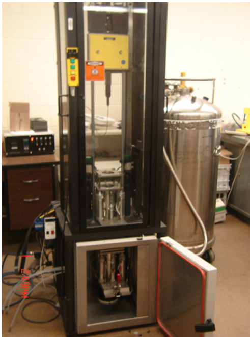
Figure 3.5 Instron Dynatup impact machine with environmental chamber.
