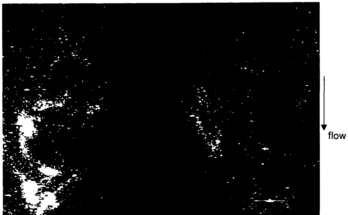
Figure 9.28: Particle flow-visualization image of the axial cross section plane of the vortex core produced by the 15° pitched semi-span wing before interaction with the shock
