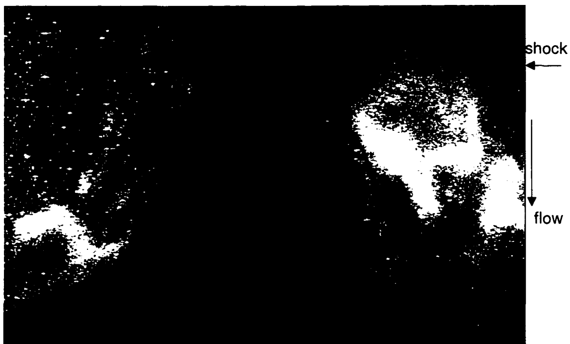
Figure 9.29 Particle flow-visualization image of axial cross section plane of the tip vortex core produced by the 15° semi-span wing after during interaction with the shock.
