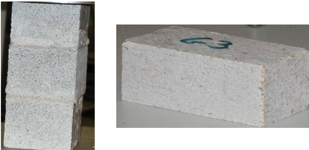
Figure 3.1: Granite stone specimens: (a) superposition of three cubic units ( 2 \times 2 \times 2 in 3 ), (b) prismatic unit ( 2 \times 2 \times 6 in 3 )
