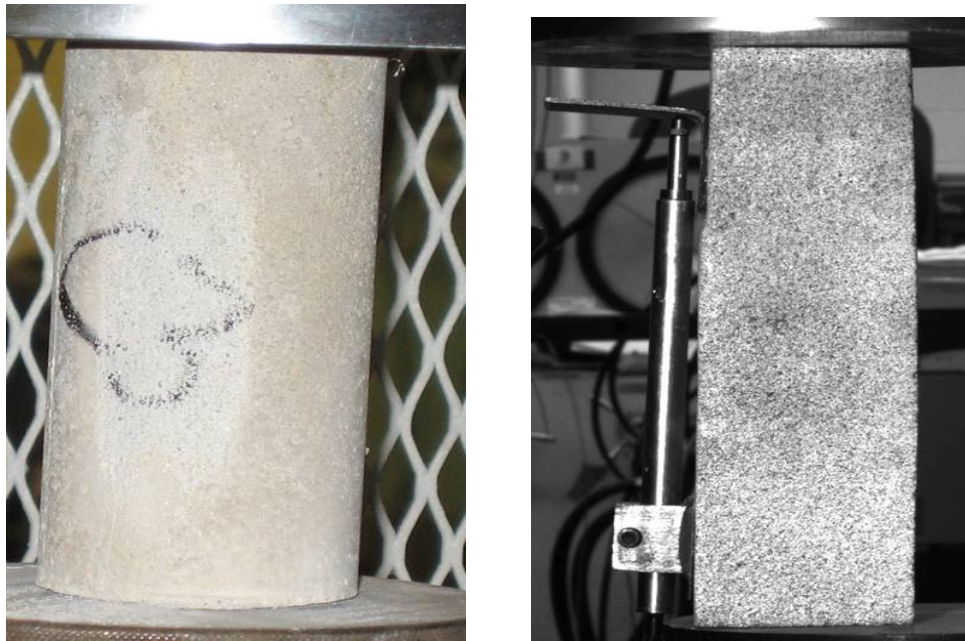
Figure 3.2: Mortar specimens: (a) cylindrical specimen with 2 in diameter and 4 in long, (b) prismatic specimen of 2×2×6 in 3
