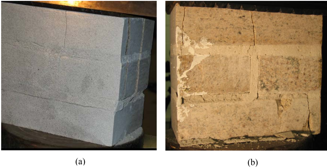
Figure 3.11 Failure modes of the granite masonry specimens under compressive loading: (a) perspective view, (b) back view
