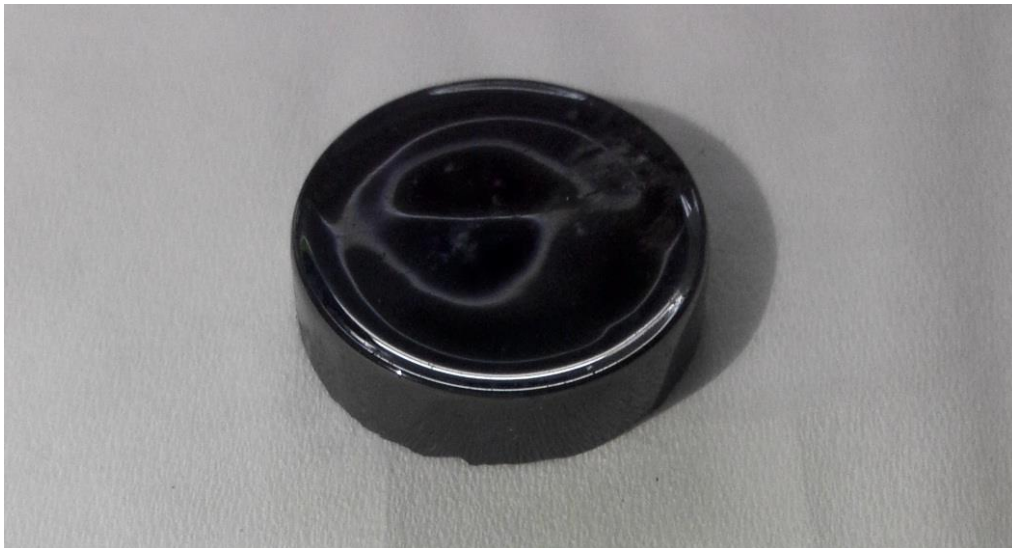
Fig. 1.5 Photo is shown above for a polycrystalline CSI ingot which was synthesized by the sintering technique.
