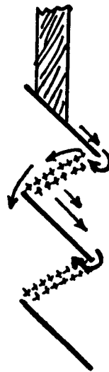
Figure 7.4-1: Steady Blow Back Sand Motion for 60° Louvers.
