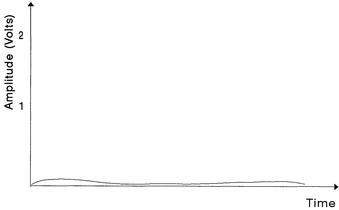
Figure.33 Steady State Signal (Absence of Vehicle)
