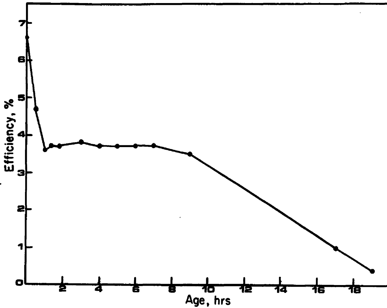
Figure 3.15 Variation of efficiency with aging time for single crystal CdSe.
