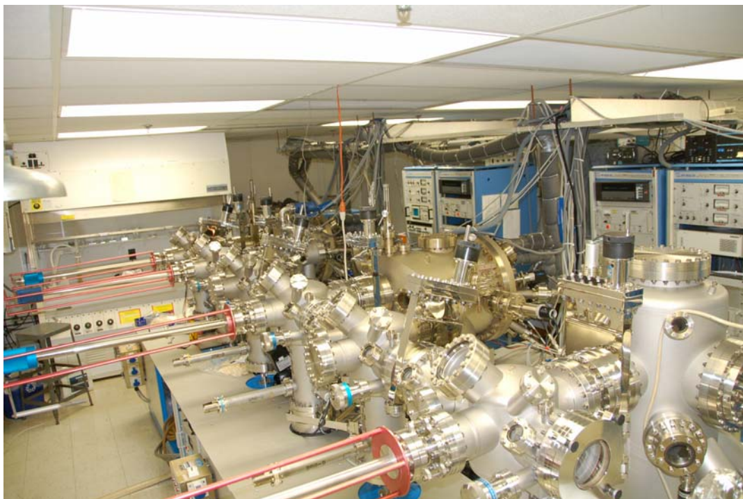
Figure 6.3: Ribier 2300P dual chamber MBE system used for growing II-VI QC structures.
