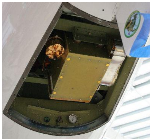
Figure 5-2. The RSP mounted on the J-31 aircraft during the INTEX-B/MILAGRO campaign (source: [Russell et al., 2007]).
