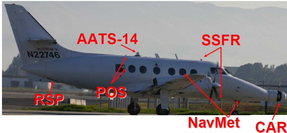
Figure 5-5. The instruments locations on the J-31 aircraft during the INTEX-B/MILAGRO campaign (source: [Russell et al., 2007]).
