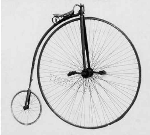
Figures 1.3 and 1.4: These two machines, built about a decade apart, illustrate the rapid innovations in bicycle technology and form. On the left, is a high-wheel bicycle produced by Overman Victory and dates from about 1886, while the image on the right is that of a safety bicycle, more specifically, an 1896 Model 41 Columbia, which includes a “drop frame” for women allowing space for a skirt to hang down. Sources: “America on the Move,” National Museum of American History, Smithsonian Institution, Negatives 811-B and 41-230.
