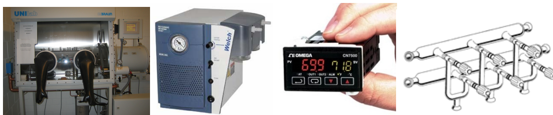
Figure 2.9 Main instruments used in the synthesis of PbTe QDs: glove box, oil-free vacuum pump, temperature controller, and Schlenk line.
