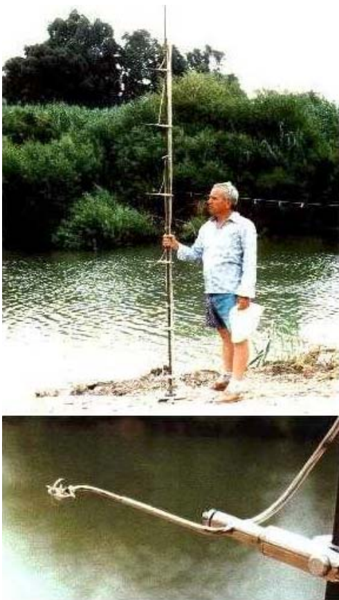
Figure 5.8: Measuring micropropeller meter and micropropeller's
