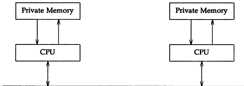
Figure 4.1: CPU's With Private Attached Memory
