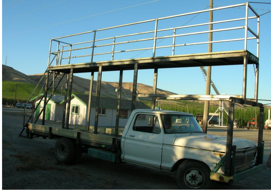
Figure A. 1 Gang-plank truck. Golden Gate Ranches, near Prosser, WA. Use of this truck provided access to the hop plant apex where we conducted Pro-Ca treatments and obtained sample collections. Treatment of hop plants using this “top down” approach enables maximum foliar application. Collection of cones from the plant apex allows for homogenous sample collection.
