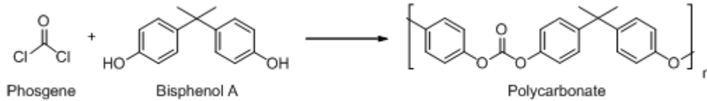
Figure 3.3 Typical synthesis of polycarbonate and structure.
