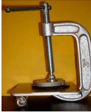
Figure 4.3 C-clamp set up from bottom up: 1) 9x9 cm steel plate, 2) Glass slide, 3) Delaminated CD-R placed face-down over glass, 4) high temperature resistant rubber layer, 5) 6 mm thick x 5 cm diameter steel plate.
