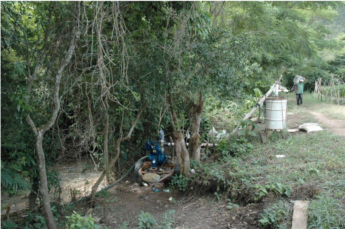
Figure 6R: A drip irrigation system. A motorized pump takes river water, the water then enters filtration barrels before being pumped into the drip lines.
