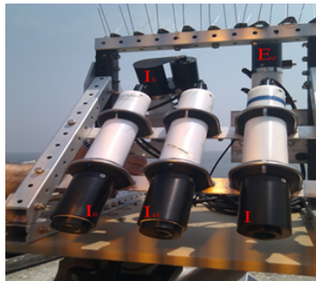
Figure 4-5. Hyperspectral radiance sensors of HyperSAS system.
